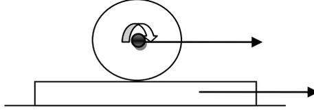
2. In the diagram shown, both the spools of thread are identical. The center of the front spool is being moved with a velocity of  $Vm/s$ . If the no slipping takes place on the ground and the tension in the string remains non zero then find out the linear and angular velocity of the rear spool. Inner radius is  $r$  and the outer radius is  $R$ .
