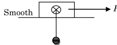
28. A homogeneous sphere, of mass  $M$ , is placed on an imperfectly rough table, and a particle, of mass  $m$ , is attached to the end of a horizontal diameter. Show that the sphere will begin to roll or slide according as  $\mu$  is greater or less than  $5(M + m)m / (7M^2 + 17Mm + 5m^2)$ . If  $\mu$  be equal to this value, show that the sphere will begin to roll.
